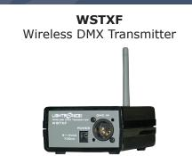
The WSTXF is a compact RF transmitter unit which transmits a DMX-512 lighting control signal to compatible receivers or wireless equipped dimmers. The input signal is received from a normal wired DMX system via a standard 5 pin male XLR connector. The WSTXF is supplied with an external power supply and a transmitting antenna.
