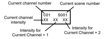
Use the ↑ and ↓ buttons to set the channel output intensity. The display shows the intensity setting as a number between 0% and 99%. A 100% setting is indicated by "FL". A "XX" setting means that the channel will be ignored for the current scene. This is useful when stacking of scenes is desired.
