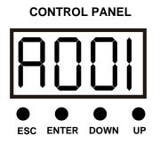
Use UP and DOWN to scroll the available choices. Push ENTER when you reach the option you want to check or set. The current setting for the option will be shown. Use UP and DOWN to change the setting. Push ENTER to invoke the new setting. Use ESC to exit from the sub menus.
