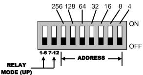
Any switch in the up position ADDS the associated value to the starting channel number. All switches down = starting channel number 1.
