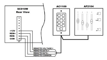
For the best results, it is advised - when installed on a large DMX data network or any network containing devices with "Master/Slave" functions such as select Lightronics FXLD or FXLE fixtures - an optically isolated splitter be installed on the output side of the SC910 in the DMX data chain.
