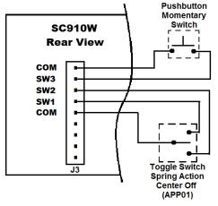
The example uses a Lightronics APP01 switch station and a typical pushbutton momentary switch. If the SC910W simple switch functions are set to factory default operation, then the switches will operate as follows:
