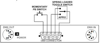
The example uses a Lightronics APP01 switch station and a typical pushbutton momentary switch. If the SC910D simple switch functions are set to factory default operation, then the switches will operate as follows:
