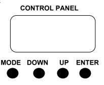
Push MODE to scroll through the available choices. Push ENTER when you reach the option you want to check or set. The current setting for the option will be shown. Push UP and DOWN until you reach the desired setting or menu then push ENTER to invoke the new setting. Push ENTER to exit from the sub menus.
