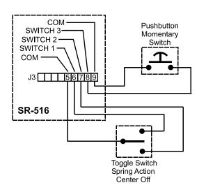
The example uses a Lightronics APP01 switch station and a momentary pushbutton switch. If the SR-516 simple switch functions are set to factory default operation then the switches will operate as follows.
