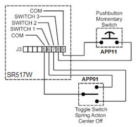
The example uses a Lightronics APP01 switch station and an APP11 momentary pushbutton switch. If the SR517W simple switch functions are set to factory default operation, the switches will operate as follows.
